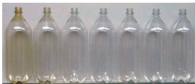
Figure 5 Two-liter blow-molded PET bottles (from Left to Right: 1200 ppm alpha-cyclodextrin, 500 ppm alpha-cyclodextrin, 200 ppm MXDA, 100 ppm MXDA, 200 ppm anthranilamide, 100 ppm anthranilamide, pure PET). [Color figure can be viewed in the online issue, which is available at wileyonlinelibrary.com .]
